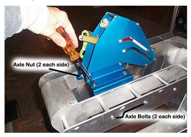
NOTE: You will need to ensure your axles extend far enough into the interior of the tread section that you can put the four slots over the axles and still attach the nuts. If your axle bolts are not long enough you will need longer ones. Axle bolts and nuts are **not** provided.
